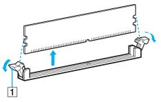
6 Grasp the memory module by the sides and remove from the computer. Store the module in a static-free bag.
